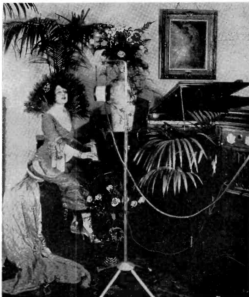
TYPICAL of the 1922 broadcast studio is this photograph taken at WJZ Newark. The artist is unknown. The microphone is of the Westinghouse "condenser" type much used at the time.
